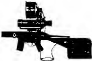
Fig. 62: Infrared scope mounted with telescopic sight mount
